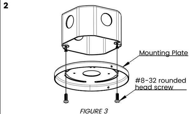
Remove Screws from the canopy assembly to release the mounting plate. Cover plate can be rotated by loosening the collar screw.
